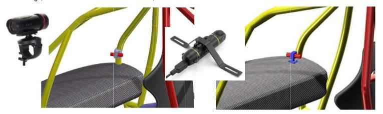
Only « Pen » type cameras will be accepted outside the car, positionned inside the perimeter of the car. Fixation must be from a mechanical type, and if a support is needed, it cannot exceed 40 mm height. Control unit must be fixed on the floor, behind the seats for touring cars or under the seats for the twin seaters.
