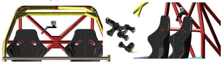
For « Pen » type cameras, it can be mounted on the front upright of the roll cage, the control unit must be fixed on the floor, behind the seats.
