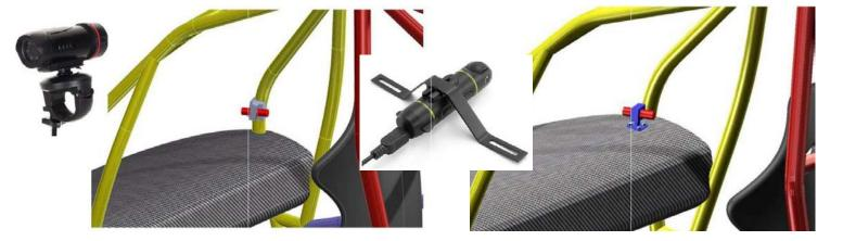
Only « Pen » type cameras will be accepted outside the car, positionned inside the perimeter of the car. Fixation must be from a mechanical type, and if a support is needed, it cannot exceed 40 mm height. Control unit must be fixed on the floor, behind the seats for touring cars or under the seats for the twin seaters.
